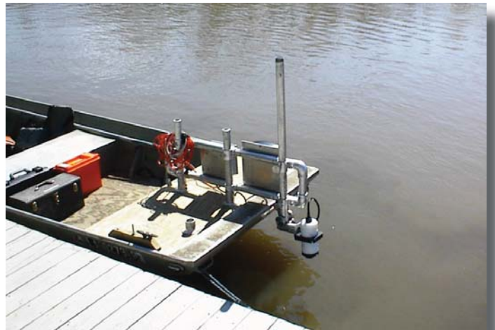
A boat-mounted ADV allowed Erick Swenson and his colleagues to conduct cross-channel transects at four depths, exploring differences in water movement at four depths and across channels. The team developed rating curves using the transect data and USGS synoptic data.
