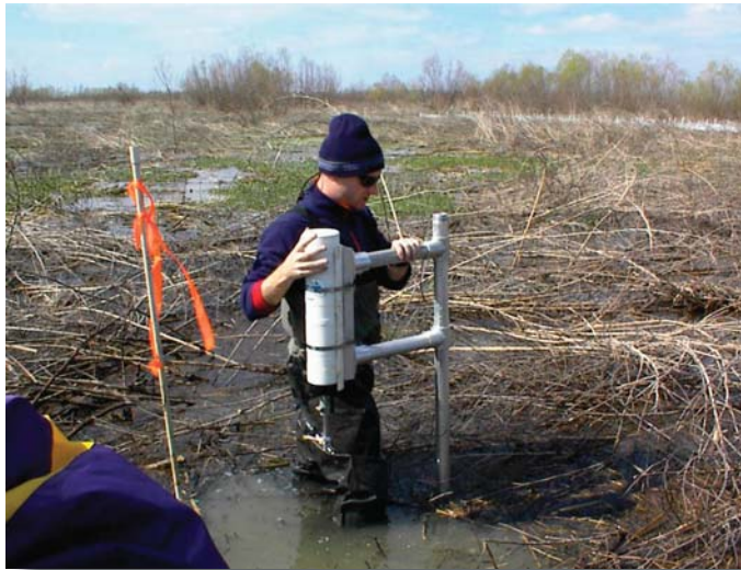
Gregg Snedden of Louisiana State University reads an acoustic Doppler Velocimeter (ADV) to measure the flow of water across the surface of a Louisiana marsh.
