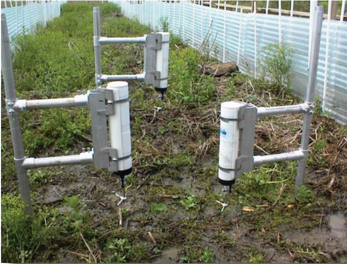
A flume built for a study on nutrient uptake shelters three ADVs that LSU scientists used to study the movement of water and sediment through Louisiana's Caernarvon Diversion. Pulse-coherent technology offers highly accurate readings even in extremely shallow or slow-moving water.
