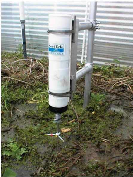
Slow-moving systems have long been a challenge to study. ADVs allow researchers to collect data on three-dimensional movement.
