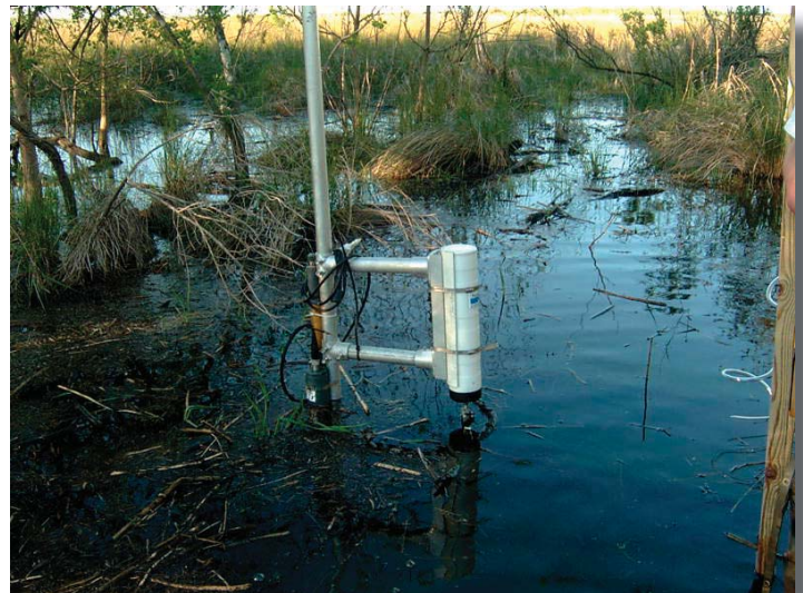
This LSU station utilized an Argonaut ADV, a YSI 6920 sonde, and a YSI 6000 OMS optical monitoring system to gather data on flow and water quality. The data are invaluable tools as hydrologists and policymakers discuss how to better manage Louisiana's shrinking wetlands.
