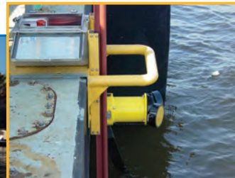
Side-Looking (Horizontal) configuration. Photo courtesy of NOAA
