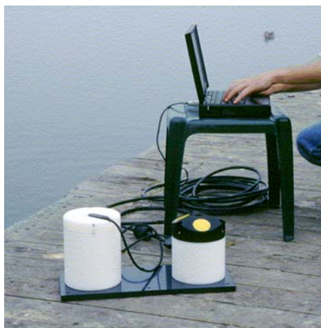
Fig 4. Autonomous Argonaut-XR system with base mounting plate
