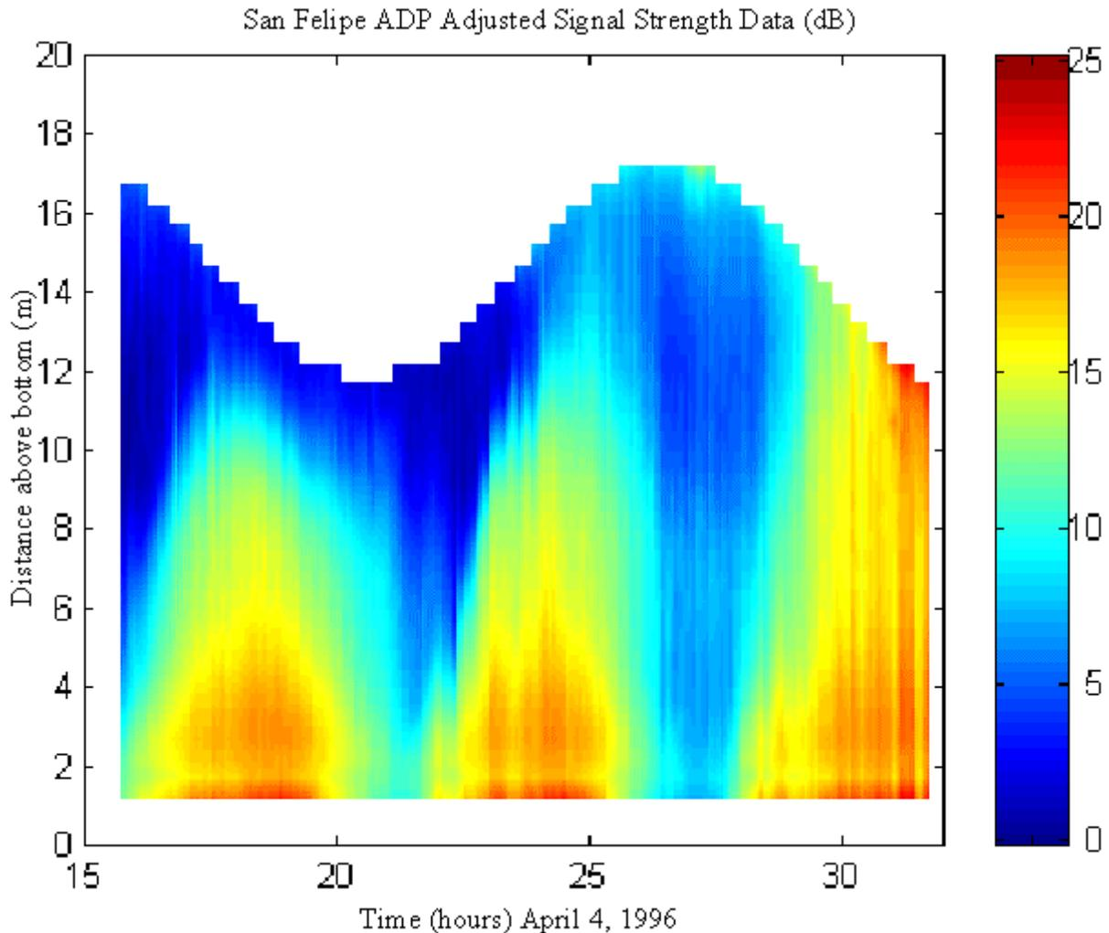
Figure 12. ADP Signal Strength Data Corrected for Range Loss
