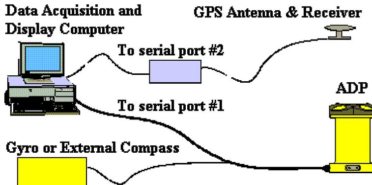
Figure 2. Operating ADP from a boat: connecting necessary equipment
