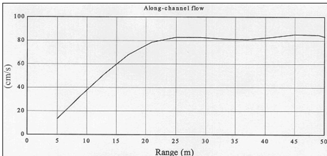
*This graph shows the actual performance of the side-looking ADP at Shinnecock Inlet, New York. Note that the main along-channel flow was reached at a distance of about 20 m from the ADP. What is astonishing here is that the ADP was submerged just 1.2 m below the surface and was able to accurately measure current data out to 50 m!*
