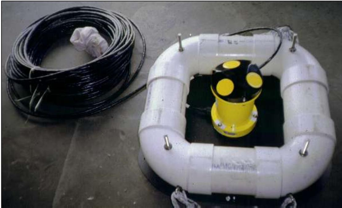
Discharge at each site is computed by first developing a relation between the mean velocity in the river (collected from discrete discharge measurements) to corresponding velocity measurements by the ADP; this technique is commonly known as "velocity-indexing". Second, a relation between water level and cross-sectional area is developed. The ADP velocity data are then used with water level data to compute continuous discharge at each site.
