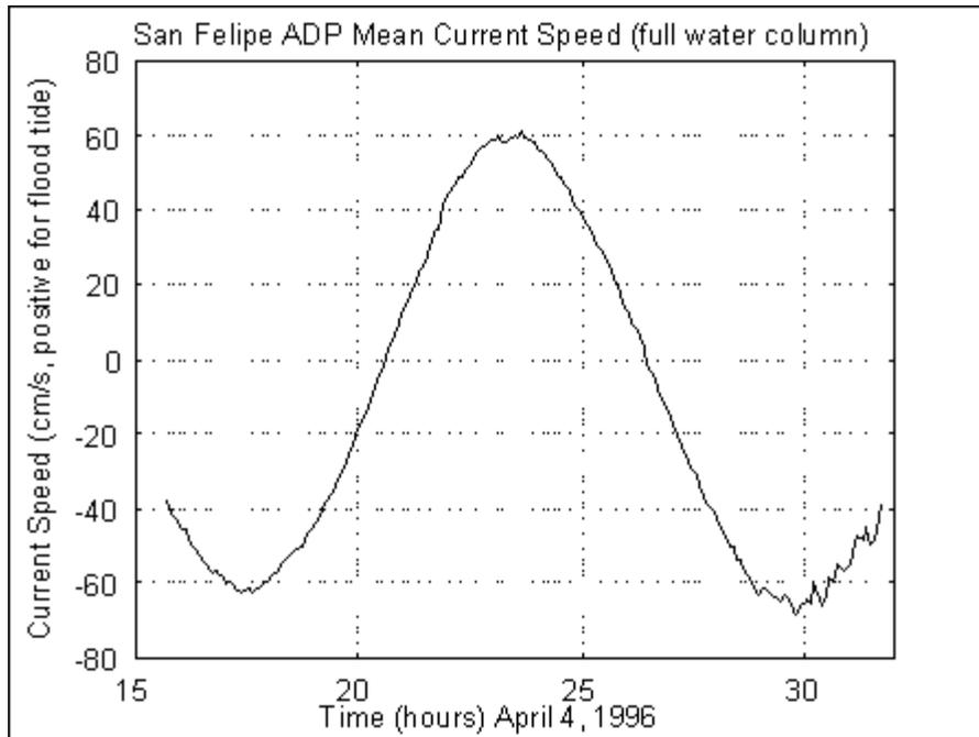
Figure 5. Mean Tidal Current Speed
