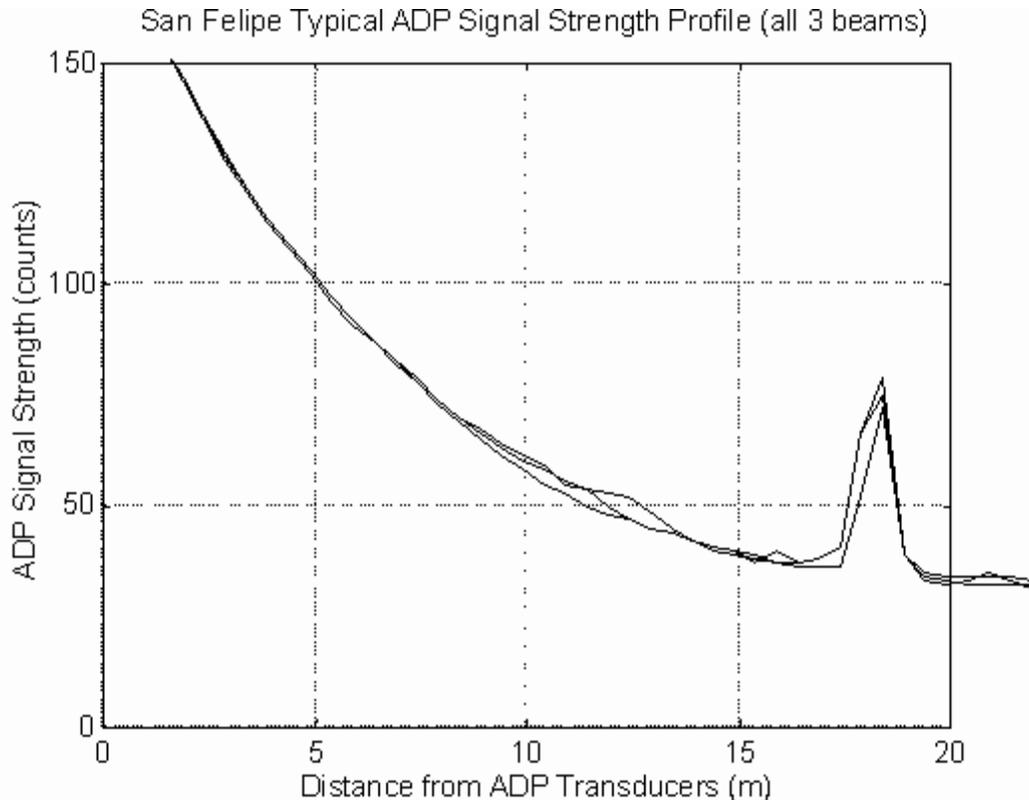
Figure 3. Measuring Surface Range using the ADP Signal Strength Profile
