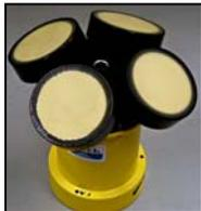
LACSD currently has 13 sites off the Palos Verdes/San Pedro shelf, all with SonTek 0.5-MHz ADPs with a Janus, 4-transducer design. Each ADP has an external, 3-battery pack canister, and a special integrated-pinger option that outputs the operational status of the system. This feature permits the status of the system to be determined without recovery - especially when there is no immediate need to service the system.
