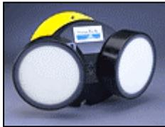
The large-diameter transducers in SonTek ADPs produce extremely narrow beams, offering distinct range advantages for horizontal profiling. Additionally, the use of a transducer shading technique minimizes side lobe interference, further increasing the maximum horizontal range of the system.
