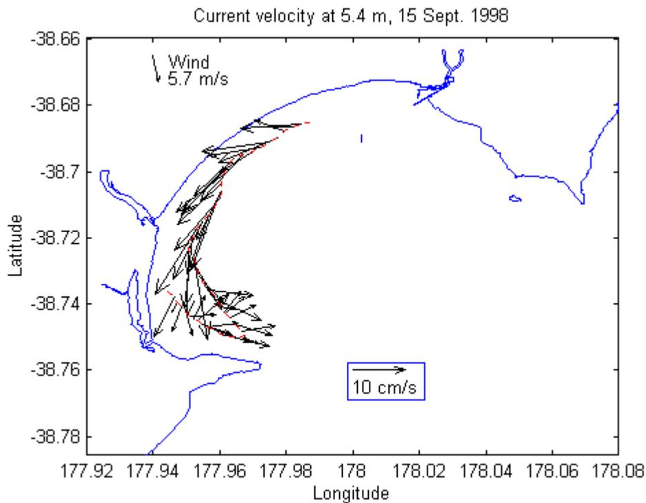
Figure 3. Currents at a depth of 5.4 m in Poverty Bay on 15 September 1998, 14:08-15:54, measured by boat-mounted ADP. A strong ( $6 \text{ ms}^{-1}$ ) offshore wind is including an associated bottom-return-flow.
