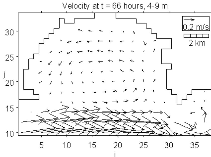
Figure 1. Numerical model velocity predictions in model layer three (4-9 m) revealing an anticlockwise circulation in response to a northeast shelf current.
