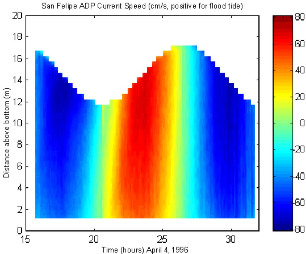
Figure 7. ADP Tidal Current Speed Contour
