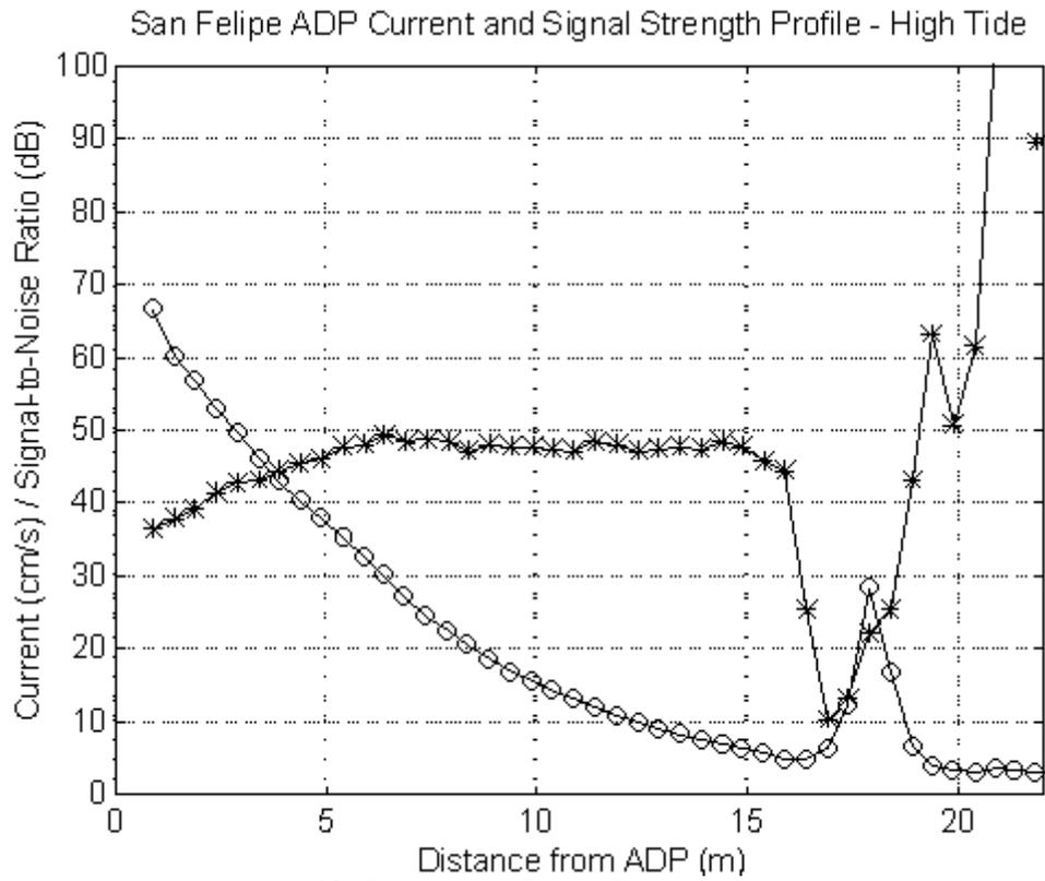
Figure 10. Current and Signal Strength (High Tide)
