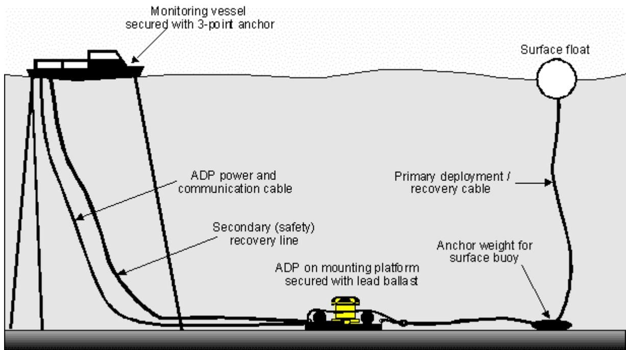
Figure 2. ADP Deployment Configuration
