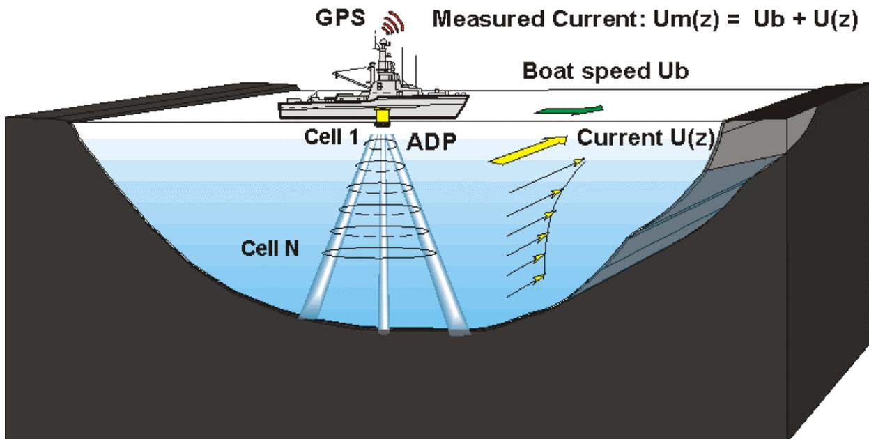
Figure 1. Measuring currents from a moving boat using an ADP
