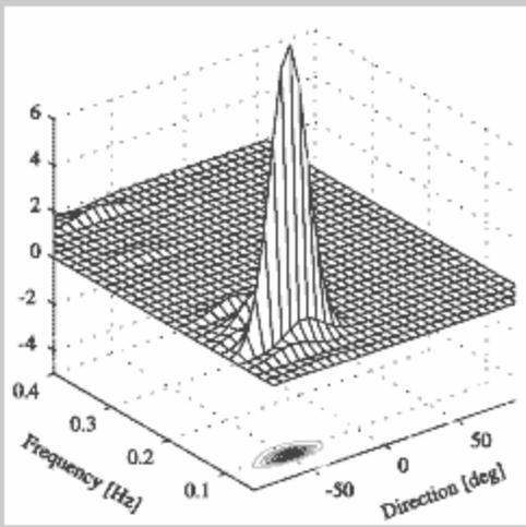
Figure 2. Directional Wave Spectrum
