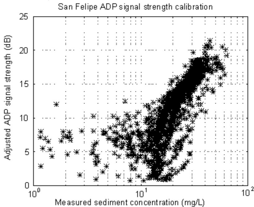
Figure 13. ADP Signal Strength Calibration using Preliminary Concentration Data
