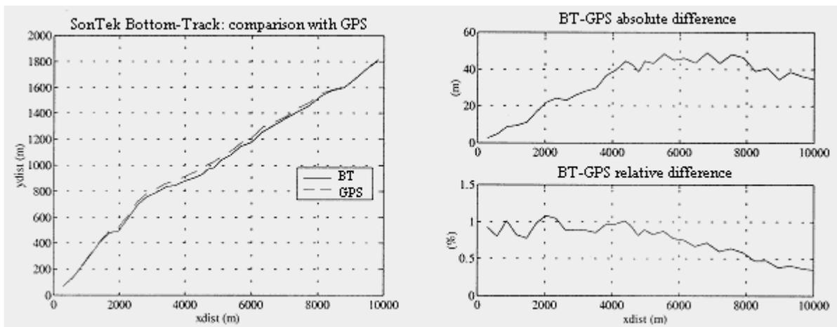
Figure 3. Field test of bottom-track vs. GPS
