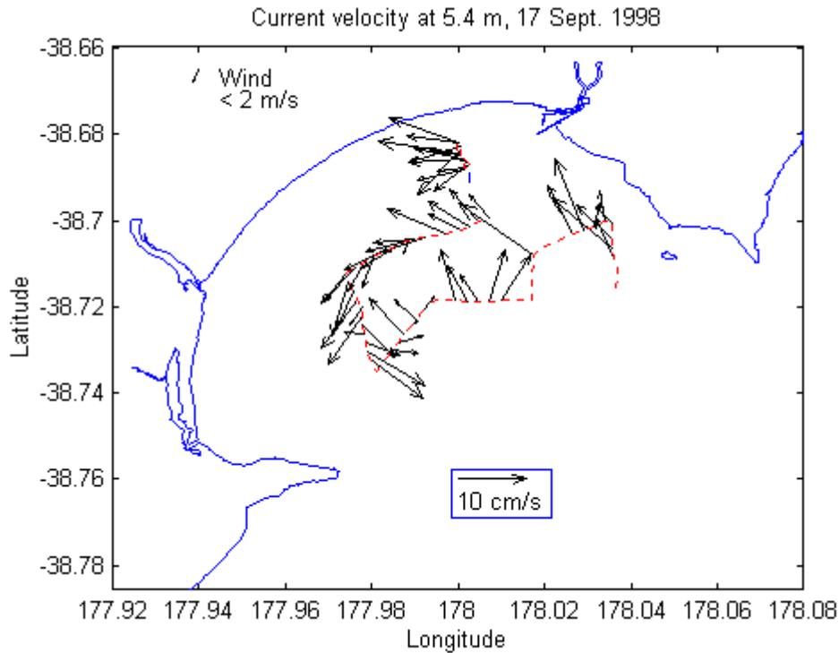
Figure 2. Currents at a depth of 5.5 m in Poverty Bay on 17 September 1998, 12:22-14:49, measured by boat-mounted, bottom-tracking ADP. Wind measured at Gisborne Aerodrome is  $1 \text{ ms}^{-1}$  from  $20^\circ$ .
