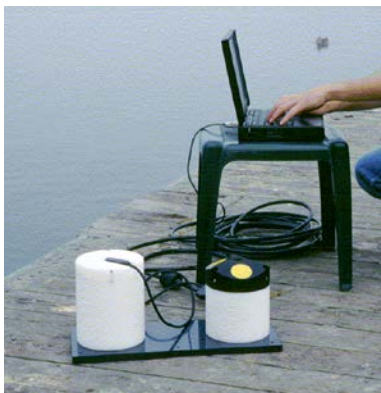
Fig 4. Autonomous Argonaut-XR system with base mounting plate
