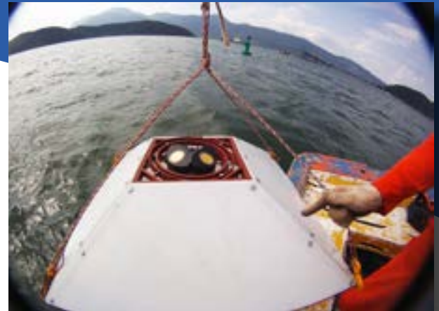
The HidroMares team deploys SonTek Argonaut-XR ADCPs—three in total—to continuously monitor currents in a forked, narrow channel in Brazil's Rio de Janeiro state. The pyramidal housing protects the current profilers from damage in the busy port.
