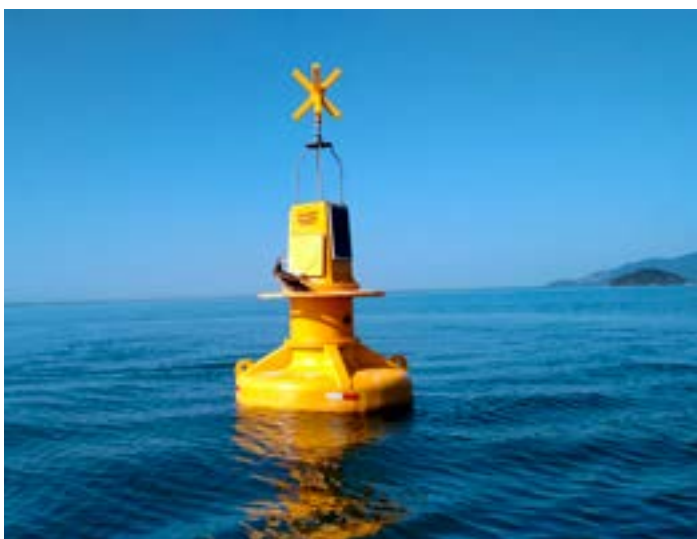
One of two Tideland buoys in the Rio de Janeiro SISMO system, with its hatch open to allow maintenance crews access to datalogging and telemetry equipment.
