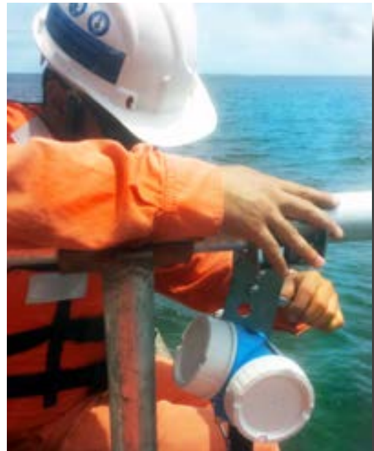
A HidroMares technician prepares a YSI Nile 502 radar water level sensor, part of the company’s innovative SISMO® harbor monitoring system.
