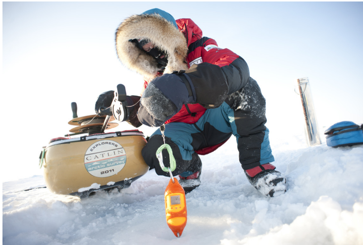
Researchers from the Catlin Survey team deploy a lightweight CTD under Arctic ice to trace effects of melting ice and warmer temperatures.
