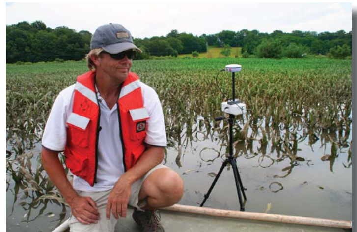
John Sloat of SonTek/YSI field tested the RTK capabilities of SonTek’s new RiverSurveyor system as he and colleagues studied floodwater behavior across the river channels and floodplains.
