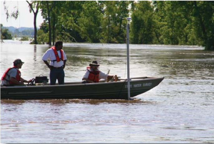
Deploying the new RiverSurveyor ADP – even activating its RTK system – during the 2008 Mississippi River flood was simple. (From left) Jim Slowikowski, Muthia Radhakrishnan and Art Schmidt put two RiverSurveyors through their paces.
