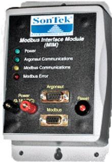
SonTek's MIM enables quick and easy integration of your Argonaut-SL/SW/XR into any Modbus-enabled system using Modbus RS-232 protocol. Acting as an RTU slave device, the MIM stores the Argonaut data in a series of specific Modbus registers so that the data can be reported to the master unit in real time.
