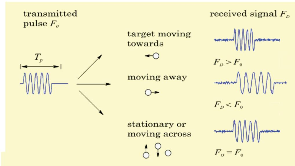
**Figure 86. Measuring target velocity with a monostatic Doppler system**
